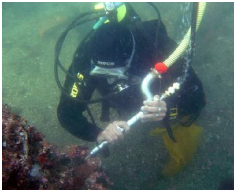
Figure 44. Pneumatic microgrinder tested in the Underwater Archaeological Park of Baiae.
